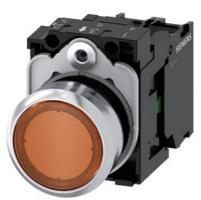
Illuminated pushbutton, 22 mm, round, metal, shiny, amber, pushbutton, flat, momentary contact type, with holder, 1NO, LED module with integrated LED 110 V AC, screw terminal, Z=20-unit packaging
