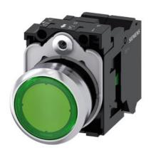
Illuminated pushbutton, 22 mm, round, metal, shiny, green, pushbutton, flat, momentary contact type, with holder, 1NO, LED module with integrated LED 110 V AC, spring-type terminal, with laser labeling, lower case
