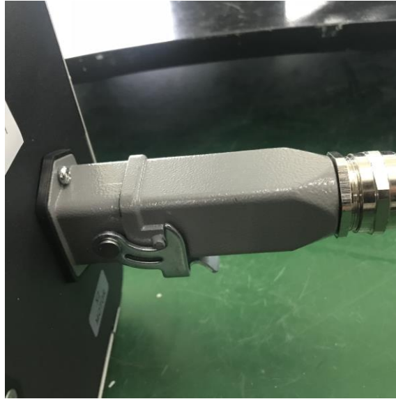
Figure 4.3 Connect controller and robot by heavy-duty cables
