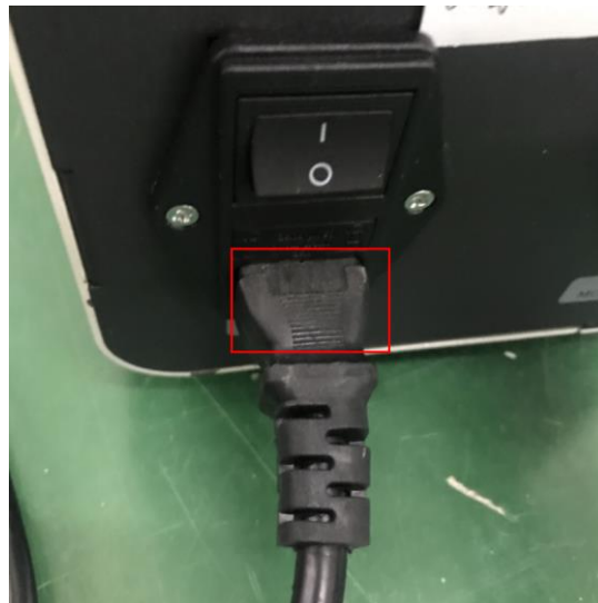
Figure 4.6 Connecting to Power Supply
