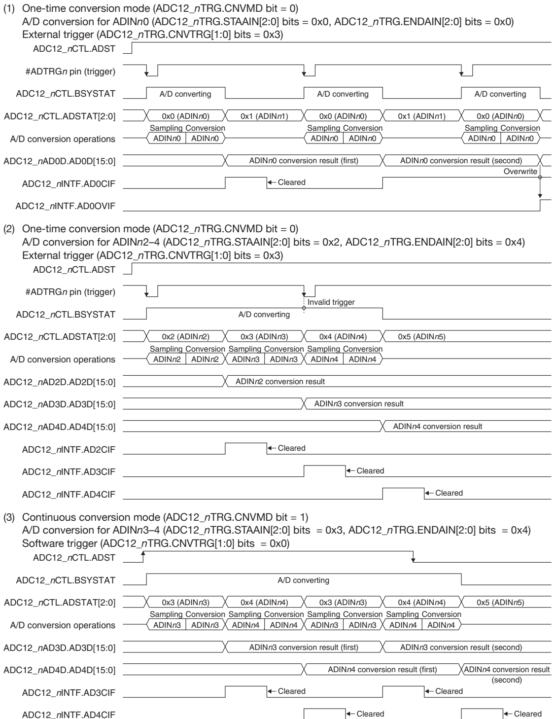
Figure 19.4.4.1 A/D Conversion Operations
