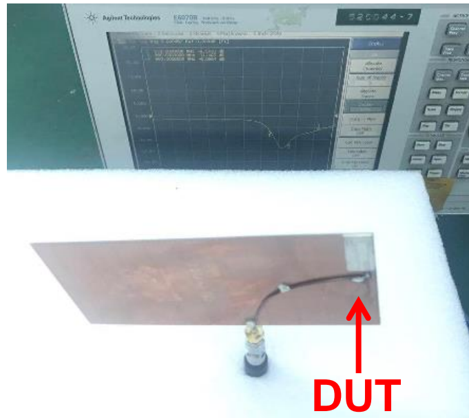
FIGURE4.1.2 ANTENNA LOADED WITH REFERENCE PCB TESTED WITH VNA E5071C
