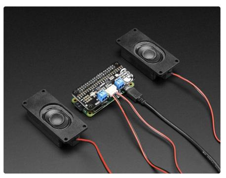
Hey Mr. DJ! Turn up that Raspberry Pi mix to the max with this cute 3W Stereo Amplifier Bonnet for Raspberry Pi. (It's not big enough to be an official HAT, so we called it a bonnet, you see?) It's the exact same size as a Raspberry Pi Zero but works with any and all Raspberry Pi computers with a 2x20 connector - A+, B+, Zero, Pi 2, Pi 3, etc. We've tested it out with Raspbian (the offical operating system) and Retropie.
