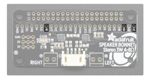
The Bonnet uses 3 data pins and they cannot be changed! Pins #18, #19 and #21 are used. All other pins are available
