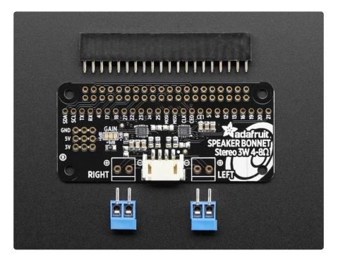
Each order comes as a fully assembled PCB with a 2x20 header and 2x terminal blocks. Some light soldering is required to attach the header onto PCB so you can plug it into your Raspberry Pi. Once that's done either plug one of our enclosed speaker sets (http://adafru.it/1669) right into the JST jack in the middle or you can solder the terminal blocks in and then connect any speaker you like.
