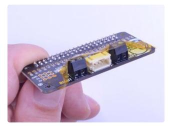
Next we will solder in the 2 3.5mm terminal blocks used to connect speakers to the Speaker Bonnet.
