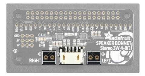
This is the fun part, you get stereo output - one left and one right channel. Each one is Bridge-Tied-Load so do not connect both outputs together to get more volume!
