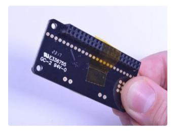
Place the 2x20 female header in so the connector is on the bottom. To make it easier to keep it in place, you can use some tape. Tacky clay also works, whatever you've got handy!
