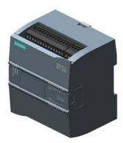
SIMATIC S7-1200, CPU 1211C, compact CPU, AC/DC/relay, onboard I/O: 6 DI 24 V DC; 4 DO relay 2A; 2 Al 0-10 V DC, Power supply: AC 85-264 V AC at 47-63 Hz, Program/data memory 50 KB
