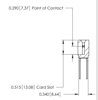
ACAD REFERENCE NO. 746 Series Ultra-Mate Card Edge Connector - Press Fit DRAWN: Part Number: 746-064-541-201 **EDAC INC** THESE DRAWINGS AND SPECIFICATIONS ARE THE PROPERTY OF EDAC INC., AND TORONTO, ONTARIO SHALL NOT BE REPRODUCED, OR COPIED CANADA OR USED AS THE BASIS FOR THE
