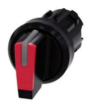
Selector switch, illuminable, 22 mm, round, plastic, red, selector switch, short, 3 switch positions I-O<II, left latching, right momentary contact type, actuating angle  $2x45^{\circ}$ , 10:30h/12h/13:30h, with laser labeling, lower case
