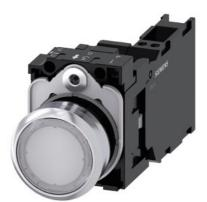
Illuminated pushbutton, 22 mm, round, metal, shiny, white, pushbutton, flat, momentary contact type, with holder, 1 NO+1 NC, LED module with integrated LED 24 V AC/DC, spring-type terminal, with laser labeling, upper case and lower case, Always upper case at the beginning of the word
