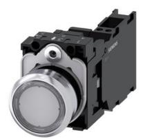
Illuminated pushbutton, 22 mm, round, Metal, shiny, transparent, pushbutton, flat, momentary contact type, with holder, 1 NO+1 NC, LED module with integrated LED 230 V AC, spring-type terminal, with laser labeling, lower case
