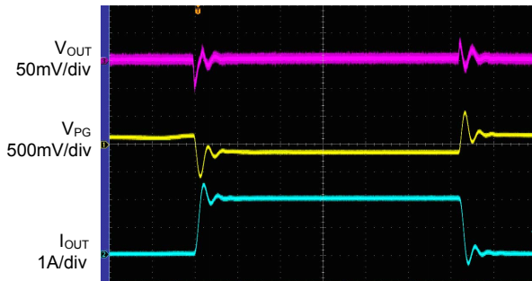
Load Transient ( V_{CTRL}=V_{EN}=5V , V_{IN}=2.2V , I_{OUT}=0 to 2A )
