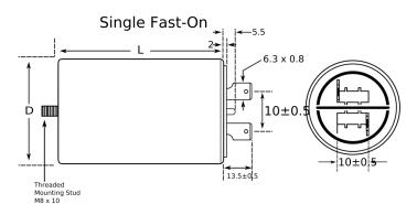
General Information Series C27 Dielectric Film/Foil Polypropylene Style Plastic Case and Cover, Ultra Sonically Welded Description Ultra Sonically Welded Seal, Safety Class PO, Features UL 94 V0 Disk **RoHS** Yes Lead Fast On (1+1) UL, VDE, UL (Construction Only), UL\_94 VO Qualifications Disk AEC-Q200 No Component 68 g Weight
