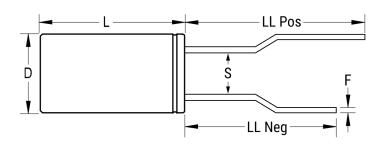
DielectricAluminum ElectrolyticDescriptionSingle Ended, Aluminum ElectrolyticRoHSYesLeadWire LeadsAEC-Q200No
