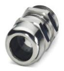
Cable gland, cable gland material: Nickel-plated brass, external cable diameter 13 mm ... 18 mm, shielding: yes, connecting thread: Pg21, color: silver, with O-ring
