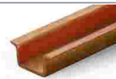
Item no.: 210-198 Copper carrier rail; 35 x 15 mm; 2.3 mm thick; 2 m long; unslotted; according to EN 60715; copper-colored www.wago.com/210-198
