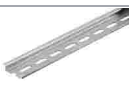
Item no.: 210-115 Steel carrier rail; 35 x 7.5 mm; 1 mm thick; 2 m long; slotted; according to EN 60715; "Hole width 18 mm; silver-colored www.wago.com/210-115
