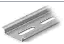
Item no.: 210-112 Steel carrier rail; 35 x 7.5 mm; 1 mm thick; 2 m long; slotted; according to EN 60715; "Hole width 25 mm; silver-colored www.wago.com/210-112
