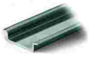
Item no.: 210-505 Steel carrier rail; 35 x 7.5 mm; 1 mm thick; 2 m long; unslotted; galvanized; according to EN 60715; silver-colored www.wago.com/210-505
