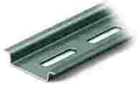
Item no.: 210-504 Steel carrier rail; 35 x 7.5 mm; 1 mm thick; 2 m long; slotted; galvanized; according to EN 60715; silver-colored www.wago.com/210-504
