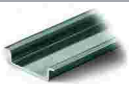
Item no.: 210-113 Steel carrier rail; 35 x 7.5 mm; 1 mm thick; 2 m long; unslotted; according to EN 60715; silver-colored www.wago.com/210-113
