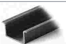
Item no.: 210-114 Steel carrier rail; 35 x 15 mm; 1.5 mm thick; 2 m long; unslotted; similar to EN 60715; silver-colored www.wago.com/210-114
