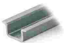
Item no.: 210-118 Steel carrier rail; 35 x 15 mm; 2.3 mm thick; 2 m long; unslotted; according to EN 60715; silver-colored www.wago.com/210-118
