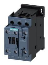
power contactor, AC-3 17 A, 7.5 kW / 400 V 1 NO + 1 NC, 230 V AC, 50 / 60 Hz, 3-pole, Size S0, screw terminal
