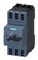
Circuit breaker size S00 for starter combination Rated current 0.5 A N-release 6.5 A Spring-type terminal Standard switching capacity
