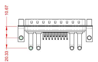
40A (CURRENT) POWER/CO-AX CONTACT RATING: (IF PRESENT) SIGNAL CONTACT CURRENT RATING: 5A PER CONTACT SIGNAL CONTACT RESISTANCE:  $10m\Omega$  MAX. **INSULATOR RESISTANCE:** 5000MΩ min. DIELECTRIC
