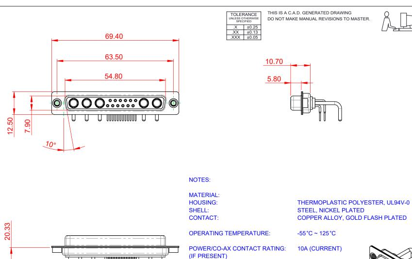
SIGNAL CONTACT CURRENT RATING: 5A PER CONTACT SIGNAL CONTACT RESISTANCE: 10mΩ MAX.
