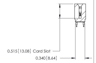
ACAD REFERENCE NO. 746-ENG MASTER 746 Series Ultra-Mate Card Edge Connector - Press Fit DRAWN: DATE: AUG 20/09 J.LEE Part Number: 746-048-560-201 CHECKED: DATE: **EDAC INC** SCALE: SHEET 1 OF 1 THESE DRAWINGS AND SPECIFICATIONS ARE THE PROPERTY OF EDAC INC.,AND TORONTO, ONTARIO SHALL NOT BE REPRODUCED, OR COPIED DRAWING NUMBER CANADA OR USED AS THE BASIS FOR THE 746-ENG MASTER MANUFACTURE OR SALE OF APPARATUS YOUR CONNECTION TO QUALITY & SERVICE WITHOUT WRITTEN PERMISSION.
