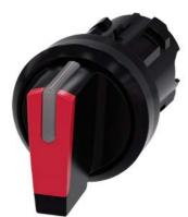
Selector switch, illuminable, 22 mm, round, plastic, red, selector switch, short, 3 switch positions I-O-II, latching, actuating angle 2x45°, 10:30h/12h/13:30h, with laser labeling, lower case
