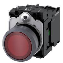
Illuminated pushbutton, 22 mm, round, plastic with metal front ring, red, pushbutton, flat, momentary contact type, with holder, 1NO, LED module with integrated LED 24 V AC/DC, screw terminal, with laser labeling, upper case and lower case, Always upper case at the beginning of the word
