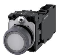
Illuminated pushbutton, 22 mm, round, plastic with metal front ring, clear, pushbutton, flat, momentary contact type, with holder, 1 NO+1 NC, LED module with integrated LED 110 V AC, screw terminal, Z=20-unit packaging
