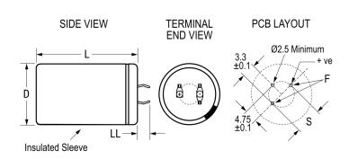
**General Information** Series ALC70 Dielectric Aluminum Electrolytic Description Snap-In, Aluminum Electrolytic RoHS Lead 3 Pin Short AEC-Q200 No Halogen Free Yes Component Weight 55 g Notes Dimensions D And L Include Sleeving. Shelf Life 156 Weeks
