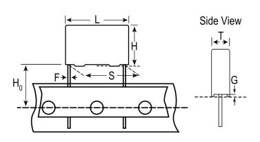
Series F881 Dielectric Metallized Polypropylene Style Radial Features MKP EMI Safety RoHS Yes Lead Wire Leads Safety Class Qualifications ENEC, UL, cUL, CQC AEC-Q200 No THB Performance No Component Weight 3.467 g Miscellaneous ClimCat: 40/110/56/B Shelf Life 104 Weeks
