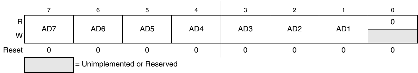
Figure 18-3. IIC Address Register (IICA)
