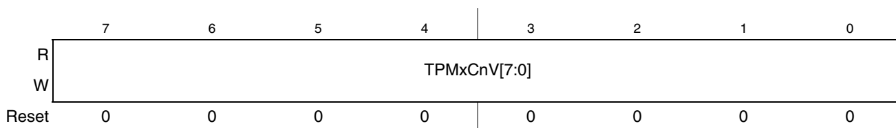
Figure 11-14. TPM Channel Value Register Low (TPMxCnVL)
