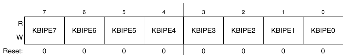
Figure 8-4. KBI Pin Enable Register
