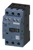
Circuit breaker size S00 for motor protection, CLASS 10 A-release 0.18...0.25 A N-release 3.3 A Screw terminal Standard switching capacity with transverse auxiliary switch 1 NO+1 NC
