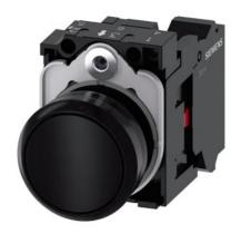
Pushbutton, 22 mm, round, plastic, black, pushbutton, flat, momentary contact type, with holder 1 NC, spring-type terminal, Z=20-unit packaging
