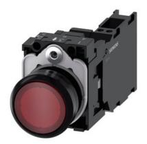
Illuminated pushbutton, 22 mm, round, plastic, red, pushbutton, flat, momentary contact type, with holder, 1 NO+1 NC, LED module with integrated LED 110 V AC, spring-type terminal, with laser labeling, inscription or symbol Customer-specific selection with SIRIUS ACT configurator (CIN)
