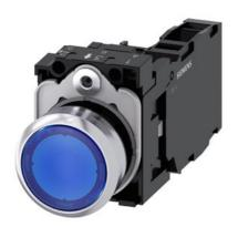
Illuminated pushbutton, 22 mm, round, metal, shiny, blue, pushbutton, flat, momentary contact type, with holder, 1 NO+1 NC, LED module with integrated LED 110 V AC, screw terminal, with laser labeling, upper case and lower case, Always upper case at the beginning of the word
