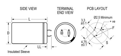
General Information Series ALC70 Dielectric Aluminum Electrolytic Description Snap-In, Aluminum Electrolytic RoHS Lead 3 Pin Short AEC-Q200 No Halogen Free Yes Component Weight 35 g Notes Dimensions D And L Include Sleeving. Shelf Life 156 Weeks
