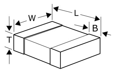
**General Information** Series VC Туре Varistors Style SMD Chip Description Surface Mount Varistors Features Low Voltage Termination Nickel Tin RoHS Yes Qualifications IEC, UL, AEC-Q200 AEC-Q200 Yes
