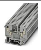
Single-level terminal block with two-sided double connection and built-in diode, cross section: 0.2 - 2.5 mm<sup>2</sup>, AWG: 30 - 10, width: 6.2 mm, color: gray
