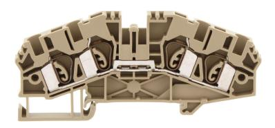
Feed-through terminal, Tension-spring connection, Mounting type: Mounting rail TS 35/7.5, Rated cross-section: 4 mm², Width: 6.1 mm, Colour: Beige
