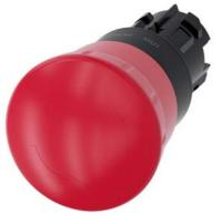
EMERGENCY STOP mushroom pushbutton, 22 mm, round, plastic, red, 40 mm, positive latching, acc. to EN ISO 13850, rotate-to-unlatch, with laser labeling, upper case and lower case, always upper case at the beginning of the word
