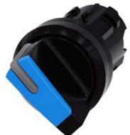
Selector switch, illuminable, 22 mm, round, plastic, blue, selector switch, short, 2 switch positions O<I, momentary contact type, Actuating angle 45°, 10:30h/12h, with laser labeling, inscription or symbol Customer-specific selection with SIRIUS ACT configurator (CIN)
