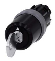
key-operated switch Siemens, 22 mm, round, plastic with metal front ring, lock number SSG10, with 2 keys, 3 switch positions I-O-II, latching, actuating angle  $2x45^{\circ}$ , 10:30h/12h/13:30h, key removal I+II, with laser labeling, upper case and lower case, always upper case at the beginning of the word
