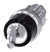
RONIS key-operated switch, 22 mm, round, metal, shiny, lock number SB30, with 2 keys, 3 switch positions I-O-II, latching, actuating angle 2x45°, 10:30h/12h/13:30h, key removal O+I, possible special locks: SB31, 421, 455, with laser labeling, upper case
