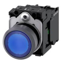
Illuminated pushbutton, 22 mm, round, plastic with metal front ring, blue, pushbutton, flat, momentary contact type, with holder, 1NO, LED module with integrated LED 24 V AC/DC, screw terminal, with laser labeling, upper case and lower case, Always upper case at the beginning of the word
