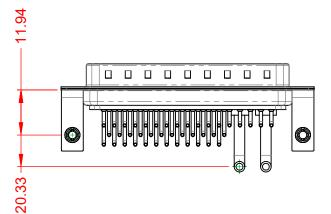
**OPERATING TEMPERATURE:** -55°C ~ 125°C 20A (CURRENT) POWER/CO-AX CONTACT RATING: (IF PRESENT) SIGNAL CONTACT CURRENT RATING: 5A PER CONTACT SIGNAL CONTACT RESISTANCE:  $10m\Omega$  MAX. **INSULATOR RESISTANCE:** 5000MΩ min.
