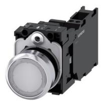
Illuminated pushbutton, 22 mm, round, metal, shiny, white, pushbutton, flat, momentary contact type, with holder, 1 NO+1 NC, LED module with integrated LED 110 V AC, spring-type terminal, with laser labeling, symbol number according to, ISO 7000 or IEC 60417
