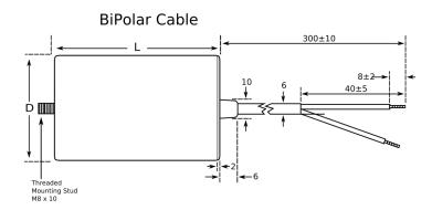
General Information Series C27 Dielectric Film/Foil Polypropylene Style Plastic Case and Cover, Ultra Sonically Welded Description Ultra Sonically Welded Seal, Safety Class PO, **Features** UL 94 V0 Disk RoHS Yes Termination Tin Copper Lead BiPolar Cables UL, VDE, UL (Construction Only), UL\_94 VO Disk Qualifications AEC-Q200 Component 50.77 q Weight
