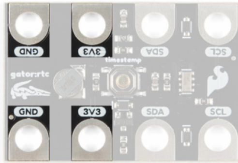
Power connection pads.
