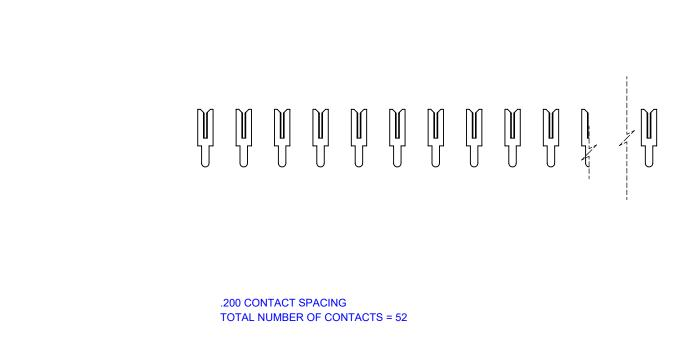
NOTE: CONTACTS ARE HELD IN A CARRIER FOR EASE OF ASSEMBLY
