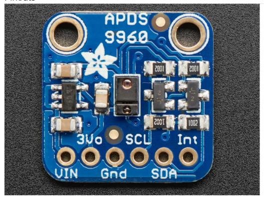
This sensor has 2 mounting holes and one header breakout strip.
