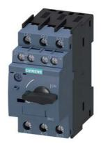
Circuit breaker size S00 for transformer protection A-release 1.8...2.5 A N release 52 A screw terminal Standard switching capacity with transverse auxiliary switches 1 NO+1 NC  $\,$
