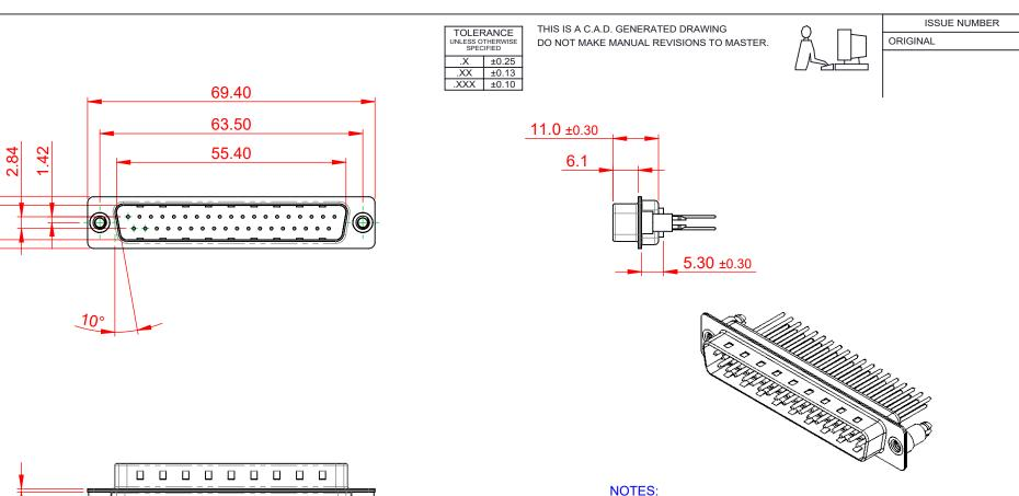
MATERIAL: HOUSING: BLUE THERMOPLASTIC POLYESTER, UL94V-0 SHELL: STEEL, TIN PLATED CONTACT: COPPER ALLOY, 30µ GOLD PLATED
