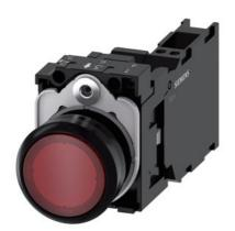
Illuminated pushbutton, 22 mm, round, plastic, red, pushbutton, flat, momentary contact type, with holder, 1 NO+1 NC, LED module with integrated LED 110 V AC, spring-type terminal, with laser labeling, upper case and lower case, Always upper case at the beginning of the word
