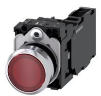
Illuminated pushbutton, 22 mm, round, metal, shiny, red, pushbutton, flat, momentary contact type, with holder, 1 NO+1 NC, LED module with integrated LED 230 V AC, screw terminal, Z=20-unit packaging
